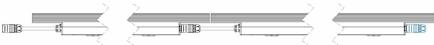
Only with a plugged-in end connector from the linea m leader cable set, protection class IP66 is achieved.
